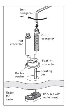
**Note:** The hot connector has 2 flat edges at the top to allow it to fit fully down and close to the top of the cold connector. Failure to do this may prevent the tap fitting onto the connector.
