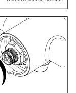
Insert 2.5mm hexagonal key into centre of cartridge spindle - Turn anti-clockwise to increase temperature.
