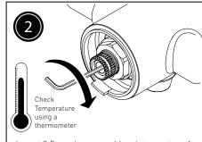
Insert 2.5mm hexagonal key into centre of cartridge spindle - Turn clockwise to decrease temperature.
