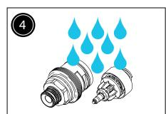
Remove Cartridge, Piston & Thermostat from shower valve body.
