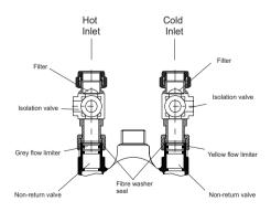
Valve inlet details as viewed from the Front of the panel when installed
