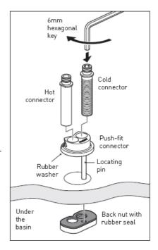
Once threading has started you can let go of the back nut. Before fully tightening the cold connector, place the 'hot connector' into the push-fit connector ensure it fits fully through the basin hole.
