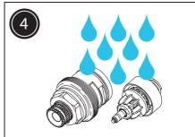
Clean Cartridge, Piston & Thermostat under cold running water (replace with Bristan parts only) and re-grease using silicon grease.
