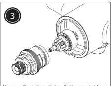
Remove Cartridge, Piston & Thermostat from shower valve body.
