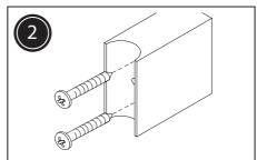
Screw the top and bottom wall brackets to the wall surface using the four long screws and wall plugs provided.
