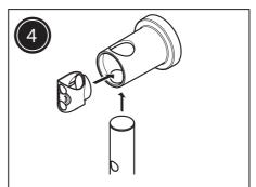
Insert the clamp and slide the rail through the top bracket.
