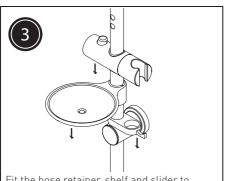
Fit the hose retainer, shelf and slider to the rail.
