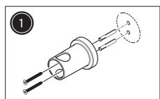
Mark the position of both wall brackets bearing in mind the height of different users. Secure the bottom bracket to the wall using fixings supplied.
