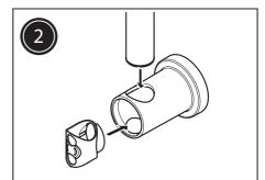
Insert the clamp and slide the rail through the bottom bracket.
