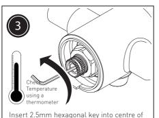
cartridge spindle - Turn anti-clockwise to
