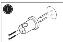
Mark the position of both wall brackets bearing in mind the height of different users. Secure the bottom bracket to the wall using fixings supplied.
