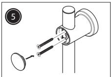
Fit the top bracket to the rail and secure in place using the fixings supplied. Fit the end caps to both brackets.
