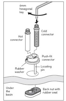
tightening the cold connector, place the 'hot connector' into the push-fit connector - ensure it fits fully through the basin hole.
