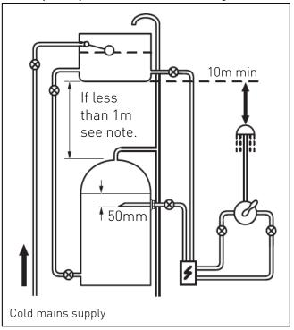
Key: Reducing Isolating Shower Pump Essex Valve Valve Flange Valve
