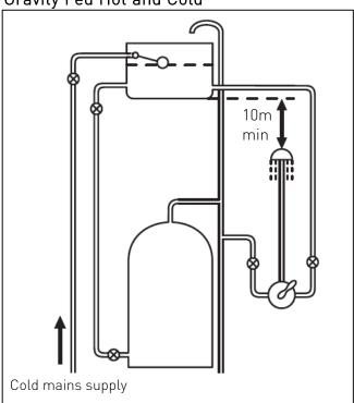
/!\ Important: If you install this shower valve with a gravity fed system, there must be a minimum head (vertical distance) from the underside of the cold water. storage tank to the showerhead position of at least 10 metres.
