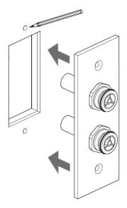
**3.** Drill suitable holes at the marked positions.
