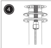
Slide 'C' shaped rubber washer and 'C' shaped metal washer onto the fixing rod up to the underside of the basin. To secure the mixer in place tighten the fixing nut onto the fixing rod until it is fully tightened against the 'C' shaped metal washer. A suitable spanner can be used to fully tighten the fixing nut.
