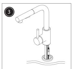
Feed the flexi tails from underneath of the basin and screw into the bottom of the mixer body by hand only (DO NOT OVERTIGHTEN). Fit the mixer body onto the plinth.
