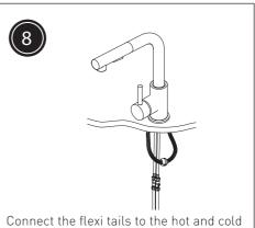
Connect the flexi tails to the hot and cold water supplies. Turn on the mains water supply and open the isolating valves using a suitable flat bladed screwdriver, letting the water flow for a few minutes to flush through the system. Check all joints and connections for any leaks.
