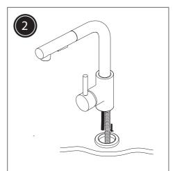
Place the plinth over the hole in the basin ensuring the washer is fitted between the plinth and the basin. Feed the hose through the hole.
