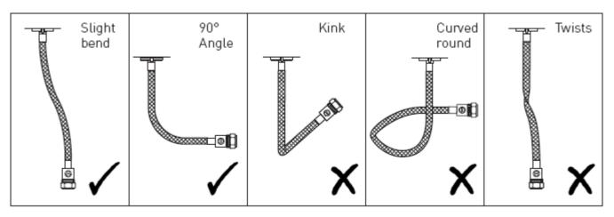
**Important:** Failure to follow these guidelines may result in poor performance and damage to the flexible connecting pipes
