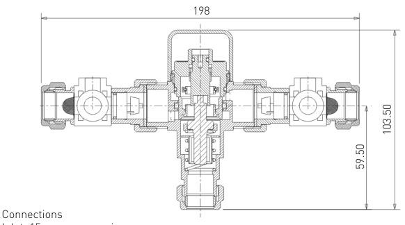
Inlet: 15mm compression Outlet: 15mm compression
