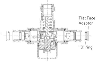
3. Insert the flat face adaptor assembly into the hot and cold inlet ports.
