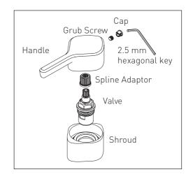
Important: Tighten the retaining nut/ valve with the correct size spanner and apply appropriate force/torque. Do not overtighten.
