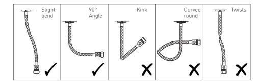
Important: Failure to follow these guidelines may result in poor performance and damage to the flexible connecting pipes.
