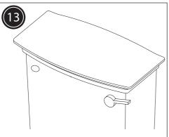
Fit the lever and place the lid onto the cistern, use cistern blanking plug to cover unuse hole.
