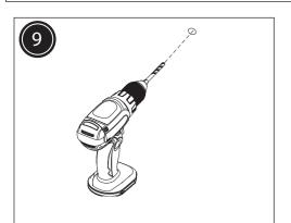
Drill fixing holes for cisten/pan through the marks on the wall/floor. Use wall plugs according to wall/ floor surface.
