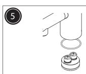
Push the mixer body onto the fixing base ensuring the rubber 'O' ring is fitted into the grove in the bottom of the mixer body. Ensure the mixer body is fitted correctly and tighten the grub screws fully to secure the mixer body in position.
