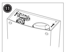
Fix the cistern to the wall with screws and washers (not supplied). Ensure the cistern is not pulled backwards, as the seal with the pan might broke.
