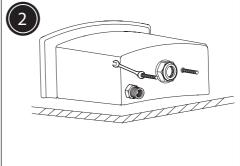
Insert fixing bolts through the holes in the cistern, using the rubber and large metal washer.
