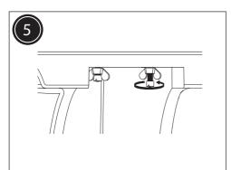
Fit the washers and wing nuts to the underside of the cistern and tighten the nuts.
