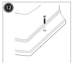
Insert screws at the base of the toilet to fix the pan to the floor using the washers provided. Do not overtighten.
