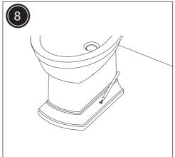
Draw a line around the base of the pan to clearly mark the position and mark the position of the screw holes.
