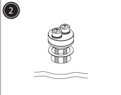
Position the fixing base into the hole in the basin ensuring the rubber washer is fitted between the fixing base and the basin.
