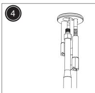
Screw the copper connecting pipes into the bottom of the fixing base by **hand only (DO NOT OVERTIGHTEN).**
