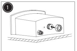
Position the cistern on its back. Assemble and insert the flush mechansim.
