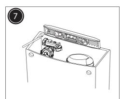
Ensure the cistern is level by placing spirit level along the back against the wall. Mark off the fixing holes through the back of the cistern.
