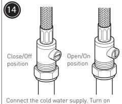
Connect the cold water supply. Turn on water supply at the isolation valve and check for leaks.
