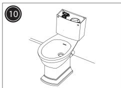
Return the pan to the desired location, make the plumbing connections and ensure that they are water tight. Ensure the pipework is flushed prior to connecting the cistern.
