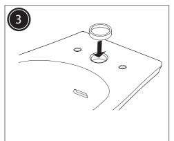
Place the large rubber gasket into the flush entrance of the pan.
