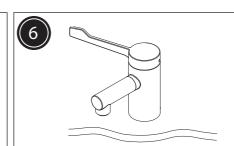
Turn on both water supplies, operate the handle in both hot and cold positions, letting the water flow for a few minutes to flush through the system. Check all joints and connections for any leaks.
