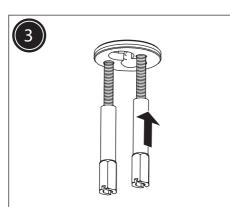
Slide the metal plate onto the threaded rods under the basin and secure the fixing base to the basin by tightening the fixing nuts onto the fixing rods. Ensure the fixing nuts are tightened fully by using a suitable spanner.
