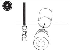
Insert a pan connector into the waste pipe.
