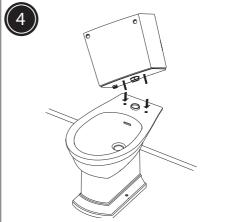
Lift the cistern onto the pan so the connecting bolt fit through the holes.
