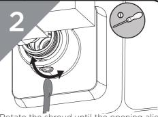
Rotate the shroud until the opening aligns with the isolation screw.
