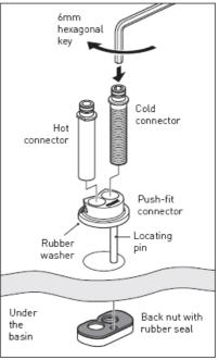
tightening the cold connector, place the 'hot connector' into the push-fit connector - ensure it fits fully through the basin hole.
