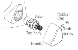
Important: Tighten the valve with the correct size spanner / socket and apply appropriate force/torque.
