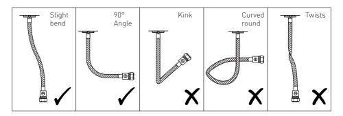
Important: Failure to follow these guidelines may result in poor performance and damage to the flexible connecting pipes.
