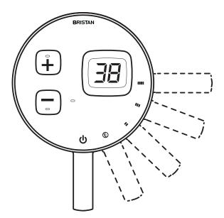
**Check Temperature controls.** Press the and temperature buttons to check that the temperature increases and decreases.
