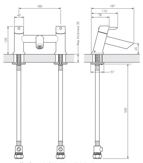
22mm Compression fitting with integral isolation valve
