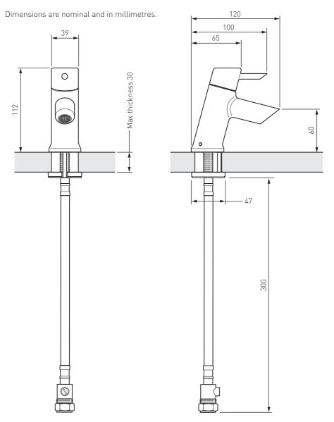
15mm Compression fitting with integral isolation valve
