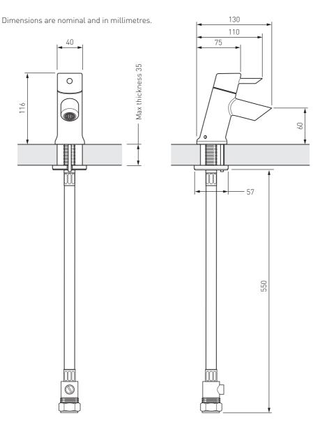
22mm Compression fitting with integral isolation valve
