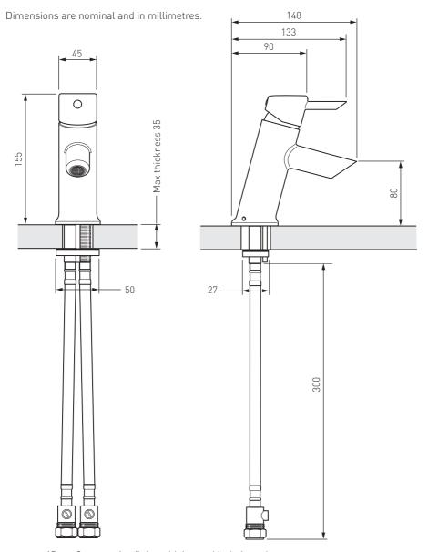
15mm Compression fitting with integral isolation valve
