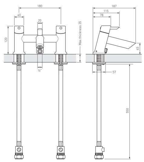
22mm Compression fitting with integral isolation valve
