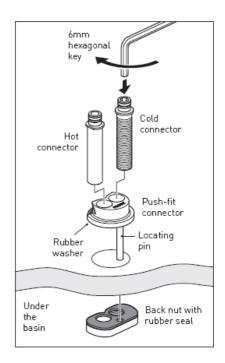
Once threading has started you can let go of the back nut. Before fully tightening the cold connector, place the 'hot connector' into the push-fit connector - ensure it fits fully through the basin hole.
