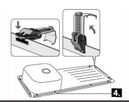
**5.** The anchor braces are designed for use with bench tops 30-40 mm thick (1). If your counter top is thinner, please insert wooden wedges between the counter top and the braces so as to secure them (2). After placing two at each corner of the sink, place the rest evenly spaced around the perimeter of the sink.
