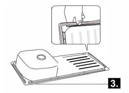
**4.** Place the anchor braces vertically and pull them up to lock into their horizontal position.
