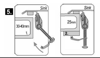
**6.** Tighten the screws of the anchor braces (with a hand screwdriver), to secure the sink in place.
