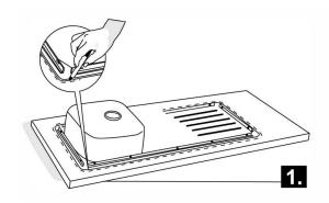
**2.** Draw another line 10 mm inside the first line. Cut a hole in the bench top following this second, inner line. (\*if the manufacturer has included a pattern in the package, then use the pattern to cut the hole in the bench top).
