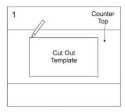
Place the cut out template onto the desired sink location. Trace around the border of the template
