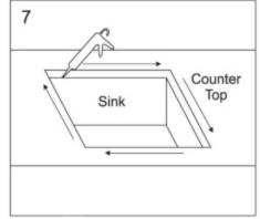
Apply suitable wet area sealant recommended for the stainless steel sink and counter top material.
