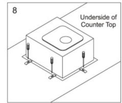
Lock the sink into the desired location. Be careful not to over tighten. Remove excess sealant.
