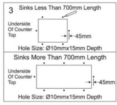
Drill into the underside of the counter top as shown in the diagram above.
