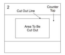
Drill into the underside of the counter top as shown in the diagram above.
