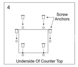
Place the fixing brackets over the screw anchor's and loosely tighten into position. Using the screws provided.
