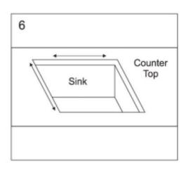
Apply suitable wet area sealant recommended for the stainless steel sink and counter top material.
