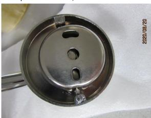
Step1 Loosen screw with screwdriver
