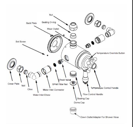
Diagrams are for illustration purposes only. Your thermostatic shower valve may superficially differ from this drawing however the installation guide steps still apply.
