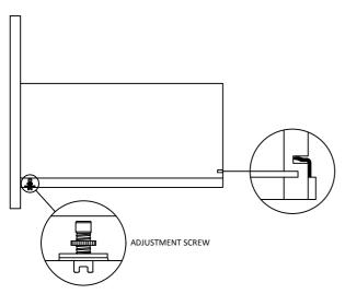
To remove drawer from cabinet, pull-out the drawer to it's full extension and gently lift the drawer box upwards.
