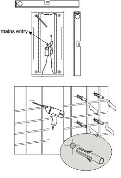
Remove the cover from the electrical connection box. Using a suitable terminal screwdriver make secure connections as follows:
