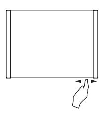
To turn illumination on or off, wave your hand under the sensor switch located at the bottom of the mirror. The heated pad will operate when the light is illuminated; The heat pad will work if the mirror lamp(s) expire. Once turned on the heating pad will warm the mirror and clear the surface of condensation.
