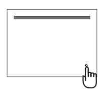
To turn illumination on touch the sensor once. To change the colour temperature, touch and hold the sensor until desired light temperature warm or cool is obtained.
