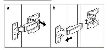
Remove the TOP door before installation. a: Lift the tab (shown) on both hinges, to release. b: Pull door back.
