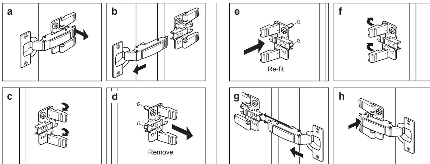
**a:** Lift tab (shown) on both hinges, to release the hinges.
