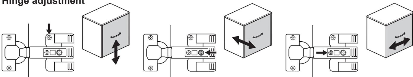
**To move door up or down:** Turn screw shown to move door up or down to suit.
