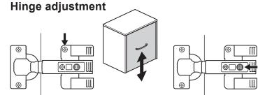
To move door up or down: Turn screw shown to move door up or down to suit.
