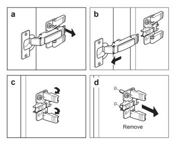
a: Lift tab (shown) on both hinges, to release the hinges. b: Pull door back. c: Lift the hinge plate tabs. d: Remove the hinge plates.
