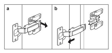
Remove the doors before installation.
