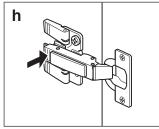
**e:** Re-fit both hinge plates on the opposite side. **f:** Fold hinge plate tabs back. **g:** Rotate door. Reposition both hinges onto the back plates. **h:** Push the front until the hinge 'clicks' into position. Attach the handle to the top set of holes on the door.
