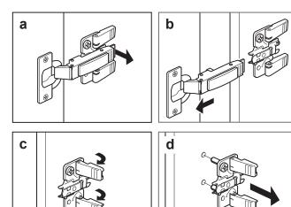
a: Lift tab (shown) on both hinges, to release the hinges.b: Pull door back. c: Lift the hinge plate tabs. d: Remove the hinge plates.
