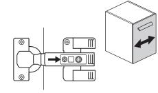
To move door left or right: Turn screw shown to move door left or right to suit.
