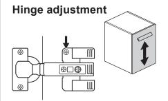
To move door up or down: Turn screw shown to move door up or down to suit.
