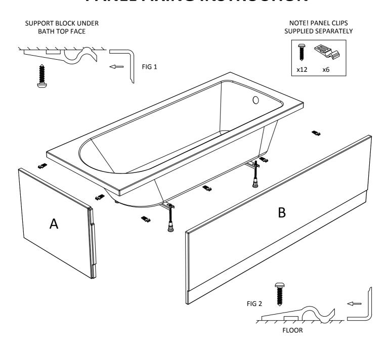
Should the cutting of panels be necessary (due to water pipes or skirting board) use a small fine toothed saw or sharp knife. Please use appropriate care and safety equipment
