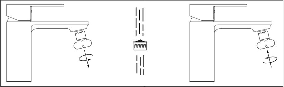
Periodically the aerator will need to be cleaned. Using an aerator key, remove the aerator from the spout, flush the aerator under water to remove the small debris or soak overnight. Re-install the aerator back into the tap and re-tighten.
