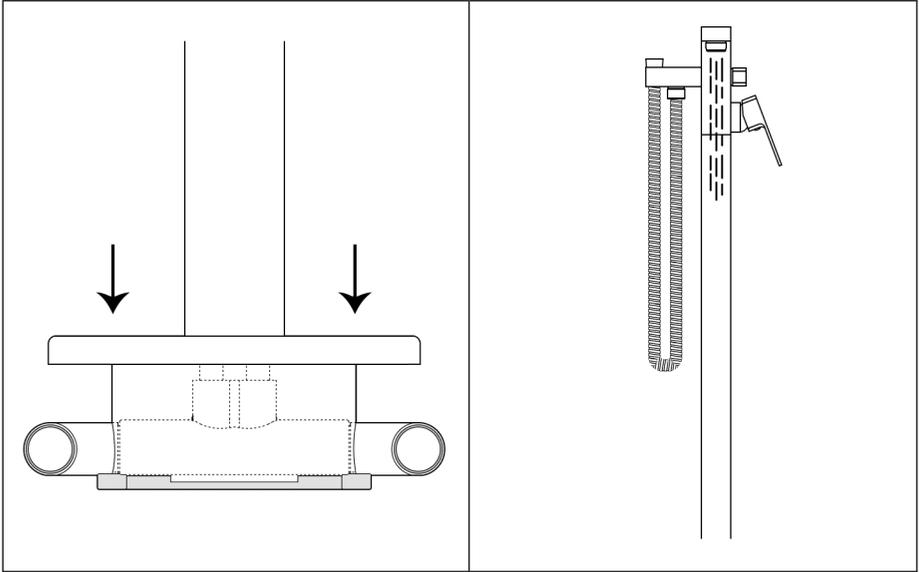
Again with great care, slide the cover plate down to cover the fixing plate and block.
