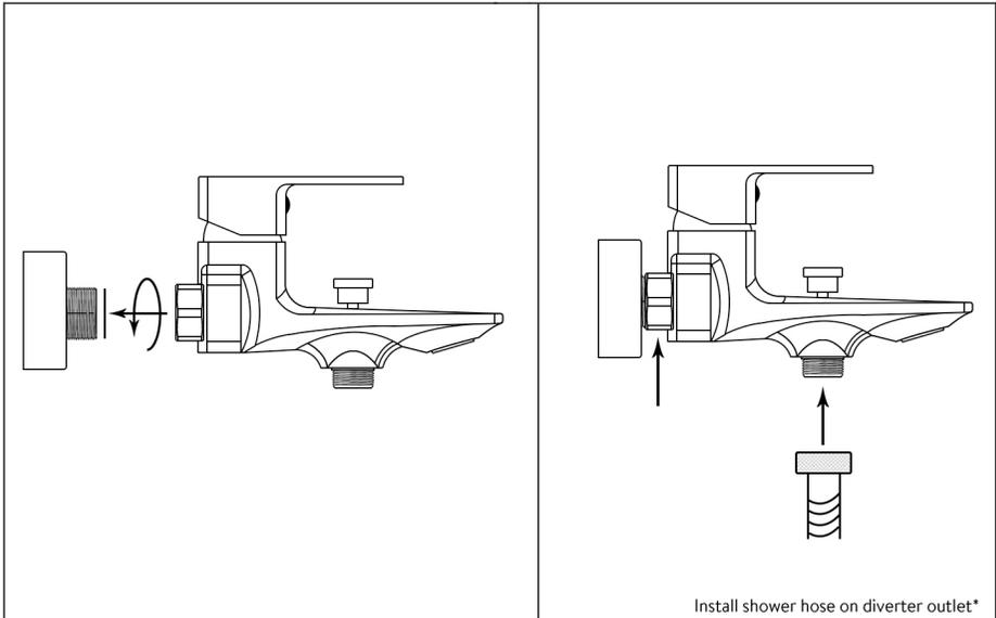
Install the washers/filters in to the mixer body, then hand tighten the mixer to the eccentrics, ensure level-ness.
