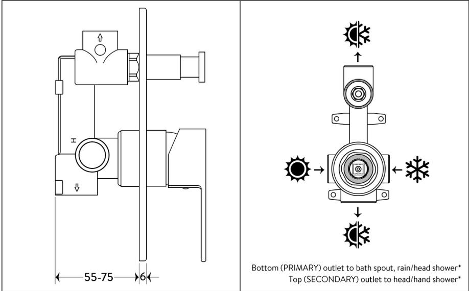
Install the concealed part at a depth so that finished surface is between the Min/Max markings shown above.
