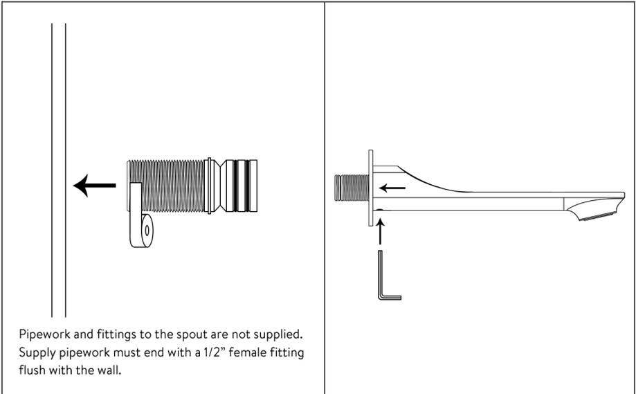
Pipework and fittings to the spout are not supplied. Supply pipework must end with a 1/2" female fitting flush with the wall.
