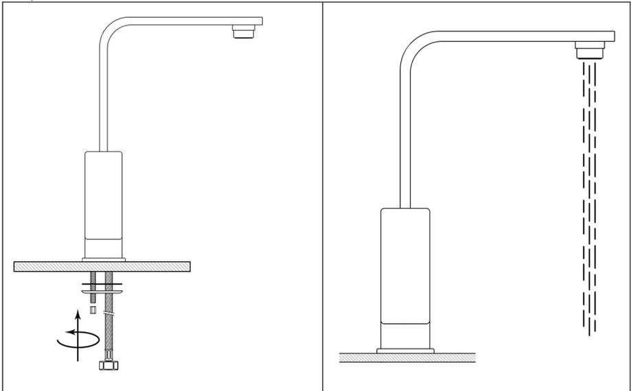
Slide the rubber 'C' washer followed by the metal 'C' washer and tighten the back nuts with a spanner to secure the mixer. Flush the pipework then connect the flexi-pipes to the isolation valves, Turn on the water, run the tap and check for leaks.
