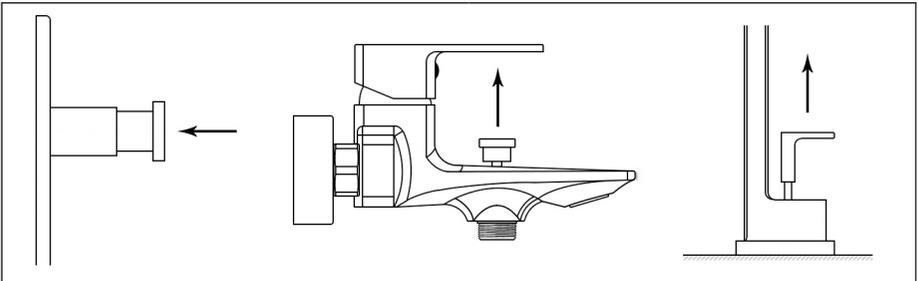
All diverters only function when the main water supply is turned on, for concealed shower valves push the button in to divert, on exposed bath/shower mixers lift the diverter button upward and for deck mounted bath/shower mixers lift the lever behind the spout.
