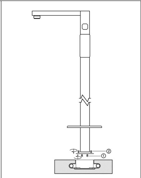
With great care, Slide the cover plate up the mixer column. Install the fixing bracket onto the bottom of the mixer column. Bolt down the mixer column to the floor block and tighten.
