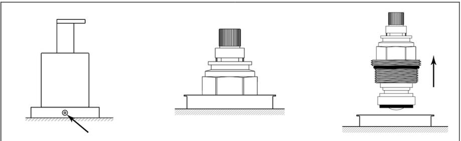
Remove the grub screw on the reverse side of the valve body and lift up. Using a spanner carefully unwind the cartridge from the valve housing. Remove, replace and re-assemble.
