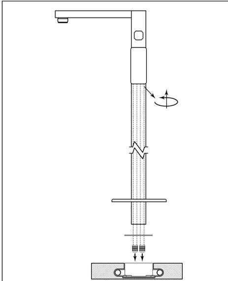
Remove the protection plugs from the block. Align the two water supplies spigots with the connections in the block. Gently push them home.
