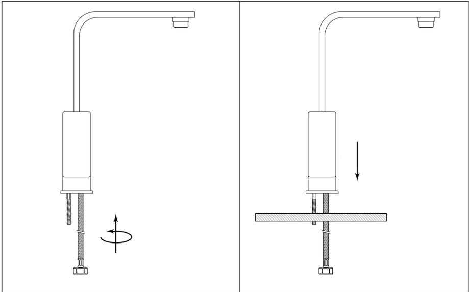
Install the threaded rods and **hand-tighten** the flexi-pipes into the bottom of the mixer body. Feed the assembly through the hole in the kitchen sink/countertop.
