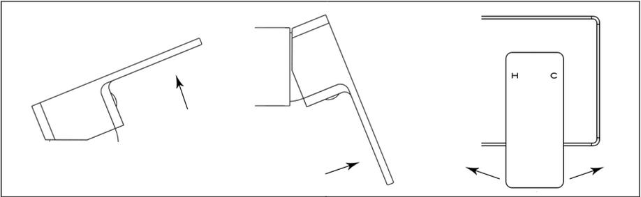
To control water flow on deck mounted mixers lift the handle upward, pull forward for wall mounted mixers. To adjust the temperature, turn the handle to the right for cold water and left for hot water.
