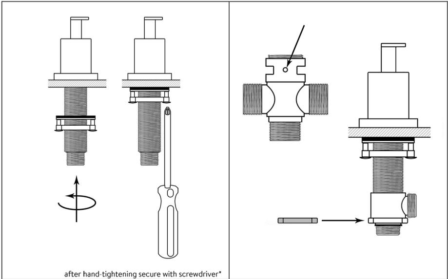
Install the components into the holes in the bathtub, from underneath place the rubber & metal washer and tighten with back nuts\*
