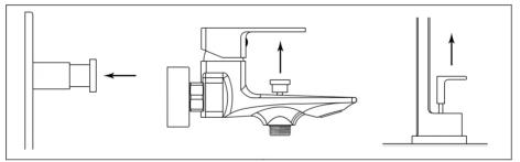
All diverters only function when the main water supply is turned on, for concealed shower valves push the button in to divert, on exposed bath/shower mixers lift the diverter button upward and for deck mounted bath/shower mixers lift the lever behind the spout.
