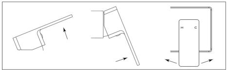
To control water flow on deck mounted mixers lift the handle upward, pull forward for wall mounted mixers. To adjust the temperature, turn the handle to the right for cold water and left for hot water.
