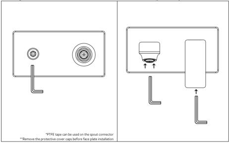
Apply the surrounding finishes, fit the face-plate onto the valve body and secure by installing the spout connector.
