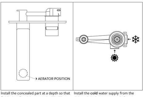
finished surface is between the Min/Max markings shown above. <u>right</u> and the **hot** water supply from the <u>underneath</u> (*if possible pressure test*).
