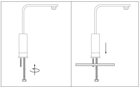
Install the threaded rods and **hand**-tighten the flexi-pipes into the bottom of the mixer body.
