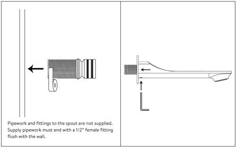
Wrap the spout connector with PTFE tape and install into the female wall fitting.
