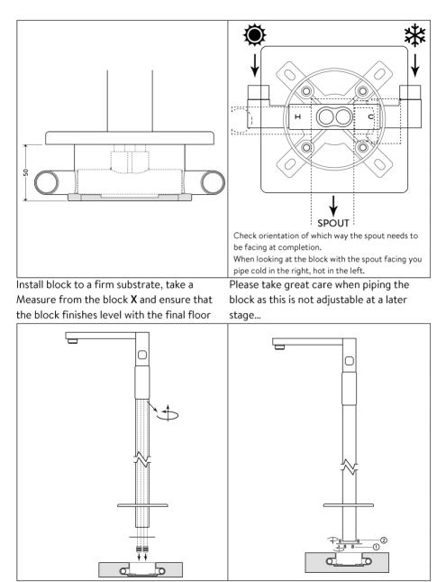
Remove the protection plugs from the block. Align the two water supplies spigots with the connections in the block. Gently push them home. With great care, Slide the cover plate up the mixer column. Install the fixing bracket onto the bottom of the mixer column. Bolt down the mixer column to the floor block and tighten.
