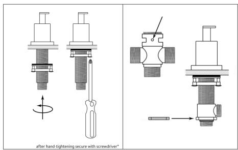
Install the components into the holes in the bathtub, from underneath place the rubber & metal washer and tighten with back nuts\* Put the connectors on the threaded bodies and secure with the 'C' clips. The spout T also requires securing with grub screw.
