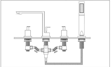
Install the 400 flexi-pipes from the valves to the spout connection T, slide the shower hose through the holder and connect to the bottom outlet of the spout T. Install the hand-shower to the shower hose. Connect water supplies to the valves, turn on and test.
