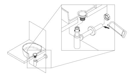
Install the bottle trap onto the waste, cut the horizontal pipe to length and install into the wall via a waste compression fitting or rubber socket.
