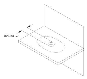
Drill waste hole allowing for the finished dimensions of the waste outlet. In this instance its  $\varnothing$ 75-110mm, please check your corresponding waste outlet product.
