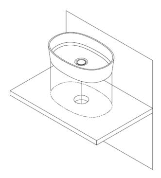
If required, place a few dots of silicon on the base of the basin, align, and place in position, allow the silicon to cure for a few hours.
