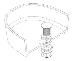
Install the waste assembly into the basin.
