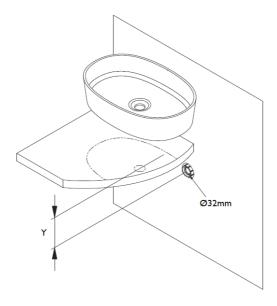
Check that the waste provision is in the correct place, check the bottle trap dimensions to ensure that the distance Y is achieveable.
