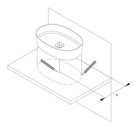
Place the basin on the countertop, take notice of the spout length of the mixer so that the distance X is correct. Mark around the perimeter of the basin and waste hole.
