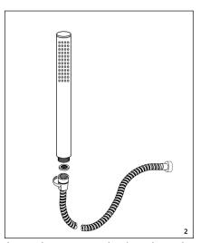
Insert the screen washer into the end of the inlet of the handshower hose. Tighten the handshower onto the hose until hand tight. Do not overtighten.
