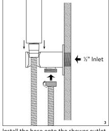
Install the hose onto the shower outlet. Use a suitable spanner to tighten the hose onto the shower outlet. Do not overtighten.
