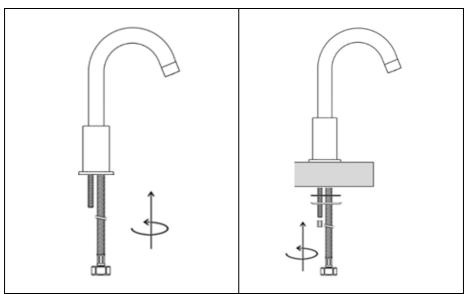
Install the threaded rod and hand-tighten the flexi-pipes into the bottom of the spout body, Position on the basin/countertop
