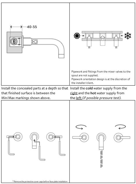
Install the face plates, then slide the spout Open the valves to test the mixer. into the spout connector, Install the handles secure all by tightening the grub screws.
