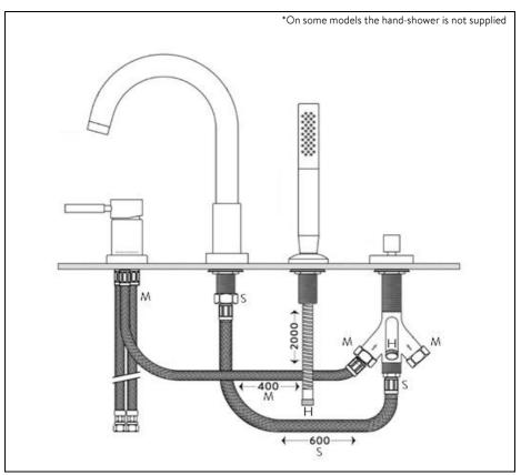
Connect the **M** flexible to either of the **M** locations on the diverter valve Connect the **S** flexible from the bottom of the diverter to the spout connection. Slide the **H** hose down through the holder and connect to the **H** outlet on the diverter
