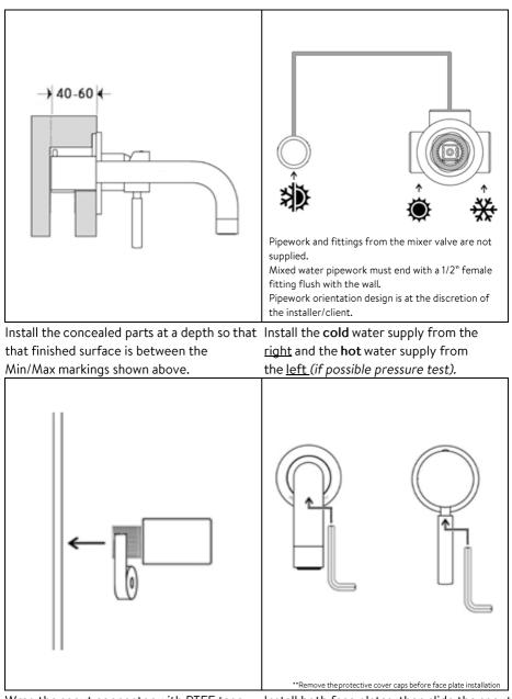
Wrap the spout connector with PTFE tape And install into the female wall fitting.
