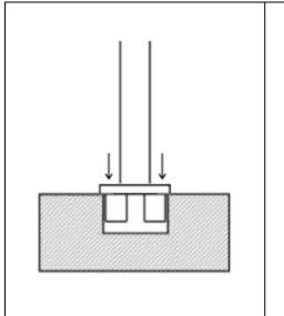
Again with great care, slide the cover plate down to cover the fixing plate and block.
