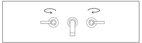
To control water flow on twin valve mixers, rotate the handles, it is always recommended that the cold valve be on the right and hot on the left. Adjust the rotation of each valve to give the temperature output you require.
