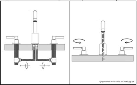
Install the Hot and Cold flexible pipes to the Flush the pipework then connect pipes corresponding valves.
