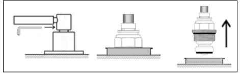
Loosen the grub screw on handle and remove, unscrew the shroud around the valve body. Using a spanner carefully unwind the cartridge from the valve housing. Remove, replace and re-assemble.
