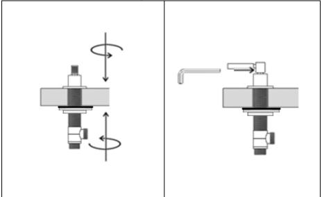
First screw the base plate and shroud onto the valve top, then from underneath tighten the back-nut up to secure.
