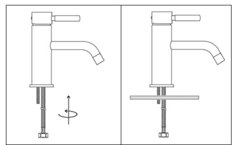
Install the threaded rods and hand-tighten the flexi-pipes into the bottom of the mixer in the basin/countertop. body.
