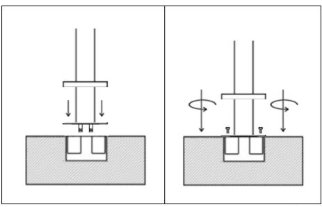
Align the two water supplies spigots with the connections in the block. gently push them home. Bolt down the mixer column to the floor block and tighten.
