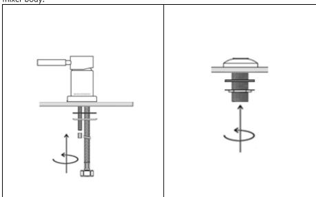
Slide the rubber 'C' washer followed by the metal 'C' washer and tighten the back nuts with a spanner to secure the mixer valve.
