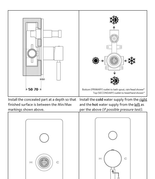
\*Remove the protective cover caps before face plate installation Apply the surrounding finishes, fit the
