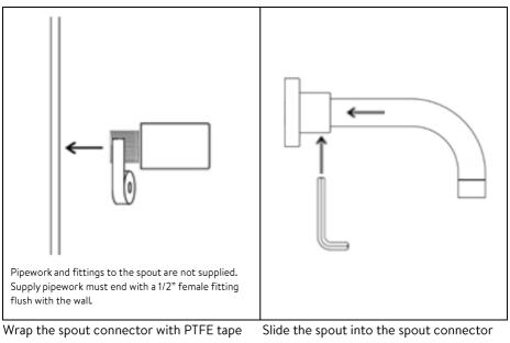
And install into the female wall fitting.
