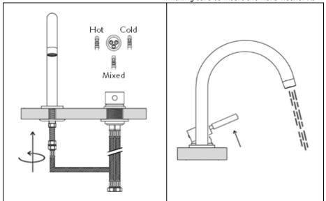
Install the mixed water flexible to the spout nut connection.
