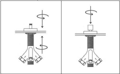
First screw the base plate onto the diverter Re-install the diverter knob. top, then from underneath tighten the backnut up to secure.
