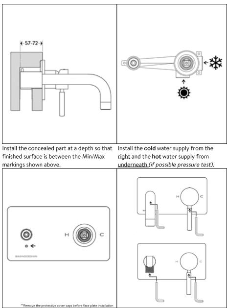
Apply the surrounding finishes, fit the face-plate onto the valve body and secure by installing the face plate screw.
