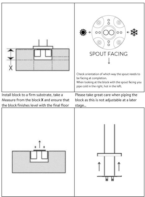
Remove the grub screws and the protection With great care, slide the cover plate up From the block. the mixer column to expose the fixing plate.
