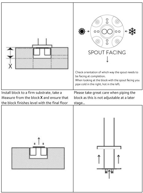
Remove the protection plugs from the block.
