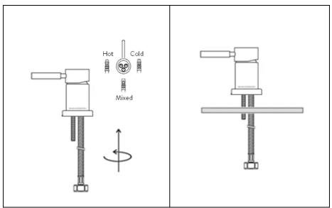
Install the threaded rod and **hand**-tighten the 3 flexi-pipes into the bottom of the mixer body. Feed the assembly through the hole in the bath/countertop.
