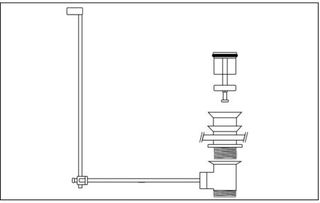
Install the waste ensuring that the foam washer is in between the waste and the basin on the top portion of the waste, the rubber washer is to be placed under the basin before the bottom part of the waste is connected and tightened up.
