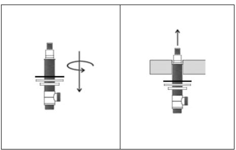
Remove the shroud and base plate from the Push the valve assembly up through the valve, screw on the back-nut, metal washer
