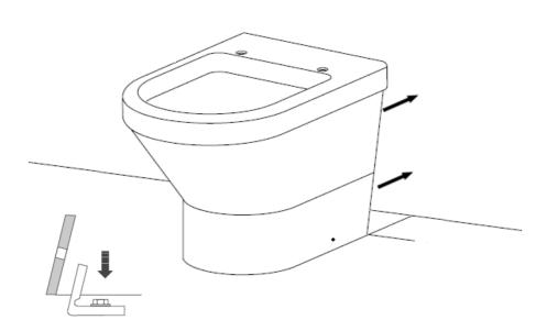
Carefully lift the WC over the fixing kit, then slide the WC backward guiding the inlet and outlet connections before fully pushing back to the wall, this should now line up with the existing drawn lines.
