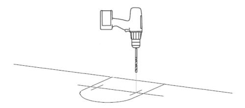
Remove the WC from position and turn over, measure the thickness of the ceramic, add this dimension across the parallel lines. Where the 2 lines meet carefully drill and plug the holes.
