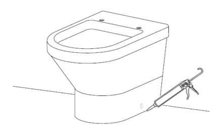
Clean away the pencil lines and place a small bead of silicon around the WC
