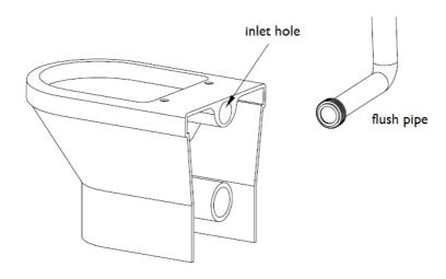
If using the WC with a concealed/furniture cistern, measure and cut the flush pipe to the required length, also make sure the waste provisions are correct. Lube all pipe connections for ease of installation.
