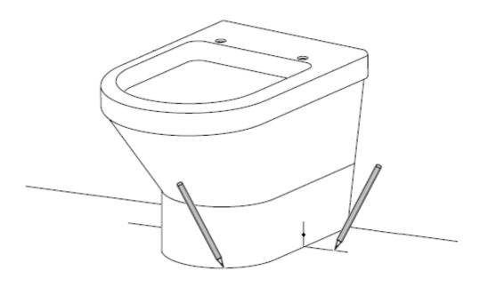
Place the WC in position and draw around the base perimeter. Also draw a line parallel to the fixing holes.
