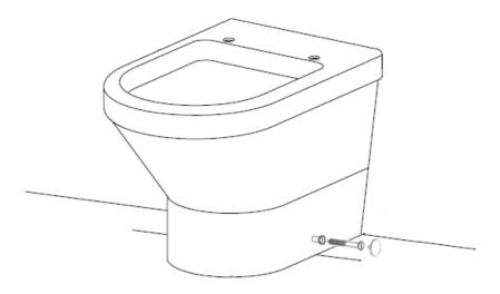
Secure the WC to the fixing kit with the plastic sleeves and the screws. Fit the plastic cover caps over the heads of the screws.
