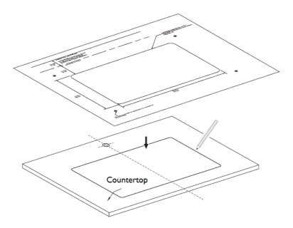
Place the cut-out template on the countertop, making sure that basin front is parallel to the front of the counter. (If no template is available use the wash basin as a template)
