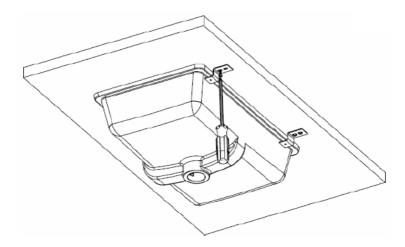
Position and align the basin with the opening, then install the brackets and tighten the screws to secure the basin. Remove any excess sealant.
