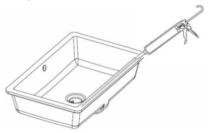
With the worktop cut and drilled, apply a bead of silicon evenly around the top flat edge of the basin.
