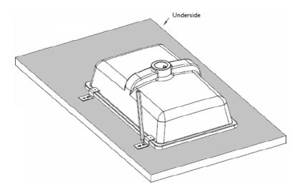
If the countertop is not fixed, to mark the brackets flip the countertop over and rest the basin in position, if the countertop is fixed use the template or hold the basin in position and mark.
