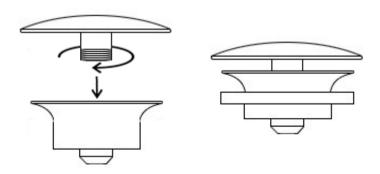
Fully hand tighten the waste top into the waste housing, then place the foam washer onto the waste housing.
