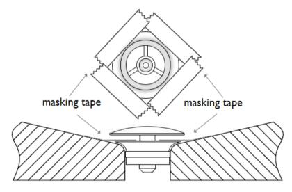
Place masking tape from the wash basin onto the waste housing, this will ensure the alignment position of the **BAGNODESIGN** logo when re-fixing waste top.
