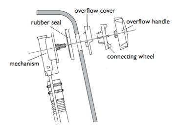
Place the rubber seal onto the mechanism and place on the outside of the bath tub, place the overflow cover on and secure with the connecting wheel, align the overflow handle and secure with the grub screw on the underside.
