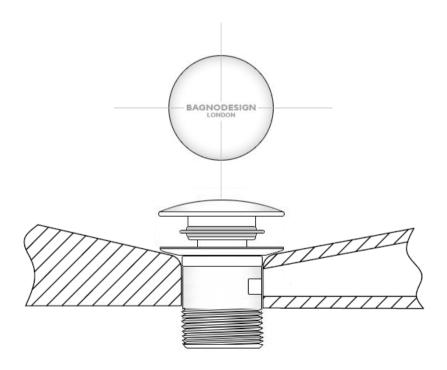
Place the waste top with foam washer into the wash basin and align the **BAGNODESIGN** logo so that it is horizontal, for wash basins with overflow, ensure that the slotted part of the waste aligns with the overflow hole.
