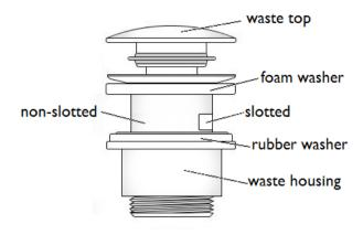
Firstly, dis-assemble the waste into its component parts shown above.
