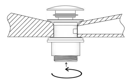
From underneath, tighten the waste housing up to the wash basin, holding the waste top during tightening will keep the **BAGNODESIGN** logo aligned.
