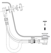
Install the overflow pipe on to the mechanism by pushing the pipe over the outlet. Install the overflow pipe into the waste connector using the compression nut and rubber olive, this connection can be cut to length to avoid creating an un-necessary trap (shown above). Make sure that at least 25mm of the overflow pipe is inserted into the waste connector then tighten.
