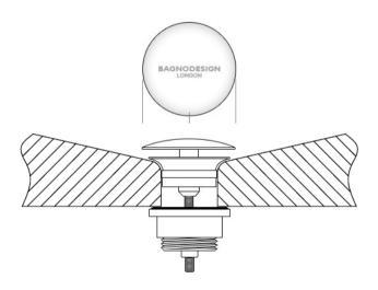
Tighten the waste top into the housing, the **BAGNODESIGN** logo will be in the previous aligned position.
