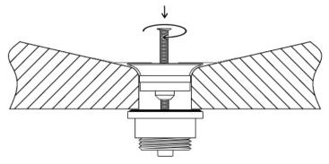
Insert the screw through the waste housing and tighten it using an allen key into the waste nut.
