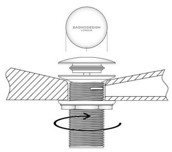
Place the waste top with 1 of the rubber washers into the wash basin and align the **BAGNODESIGN** logo so that it is horizontal, for wash basins with overflow, ensure that the slotted part of the waste aligns.
