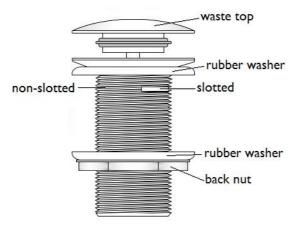
Firstly, dis-assemble the waste into its component parts shown above.
