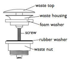
Firstly, dis-assemble the waste into its component parts shown above.
