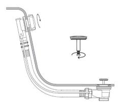
With all the items installed the mechanism can be tested, rotate the overflow handle to allow the pop-up plug to move up and down, if the pop-up plug is not high enough, it can be adjusted on the screw as shown above. If your bath waste is a combination bath filler, fit as above then connect the ½' outlet to the bath/shower mixer.
