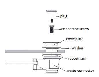
Place the rubber seal onto the waste connector and place on the underside of the bath tub place the washer in the waste hole and tighten the cover plate with the connector screw into the waste connector. Place the plug in position.
