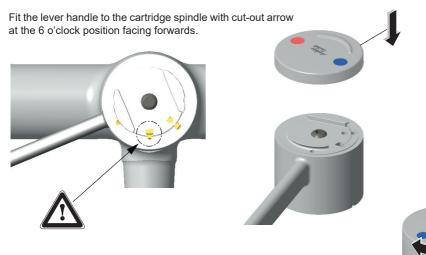
Fit the lever handle screw and tighten fully to a torque of 5 NM using a 4mm hexagon key.
