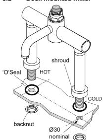
The deck mounted mixer is designed to be deck mounted on a countertop of maximum thickness 40mm
