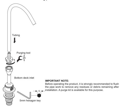
The purging kit also provides the facility to obtain water supply temperatures at the inlets.
