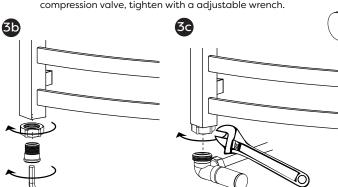
Feed the top union nut through the threaded tail, then screw the threaded tail to your chosen radiator. Secure the connection using an Alan key.
