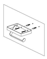
STEP 2: Fix the Screws and the expansion
