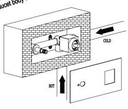
Step 5: Install the spout and handle to the correct positions.
