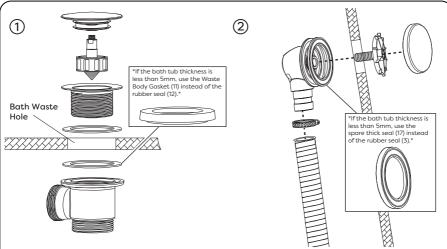
Place the rubber washer over the bath waste hole, then proceed to feed the flange through the same hole.
