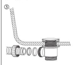
Attach the PVC hose to the waste body using the rubber seal, plastic ring, and hose nut provided. Ensure that the connection has a tight seal. **Be careful not to overtighten.**
