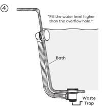
Connect the waste trap to the waste body. Turn on the water supply, fill the bath with water and check all joints to ensure there are no leaks.
