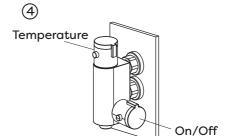
Connect the valve body with the two washers to the threaded tails on the reducers. Tighten with a adjustable wrench/spanner.
