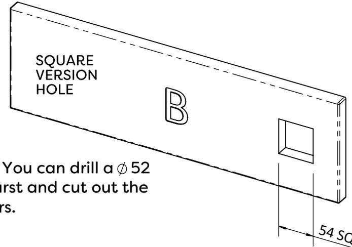
Note: You can drill a  $\phi 52$  hole first and cut out the corners.
