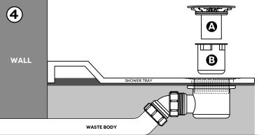
Feed the 'Inner Chamber' (B) and 'Dome Cap' (A) through the shower tray hole and connect to the waste trap.
