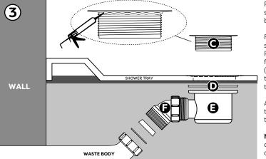
Pipe a fine bead of good quality silicone sealant around the bottom edge of the 'Flange' (C).
