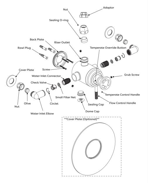
Diagrams are for illustration purposes only. Your thermostatic shower valve may superficially differ from this drawing however the installation guide steps still apply.
