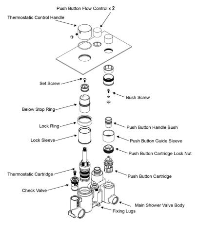
Diagrams are for illustration purposes only. Your thermostatic shower valve may superficially differ from this drawing however the installation guide steps still apply.
